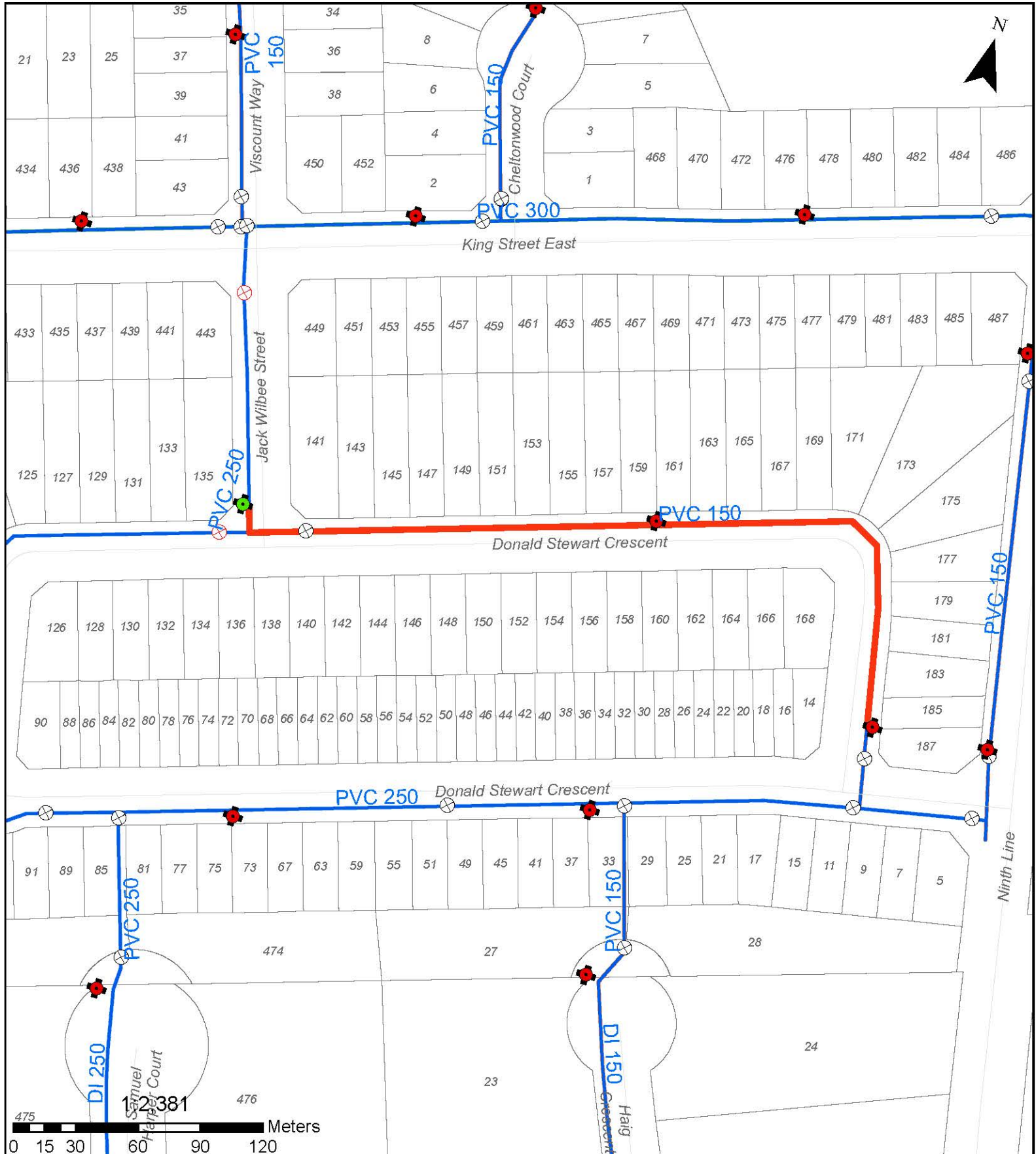
Mount Albert Water Supply System Upgrades Schedule 'B' Class EA Figure 3- C-factor Testing #2 PVC 150 mm Donald Stewart Crescent
