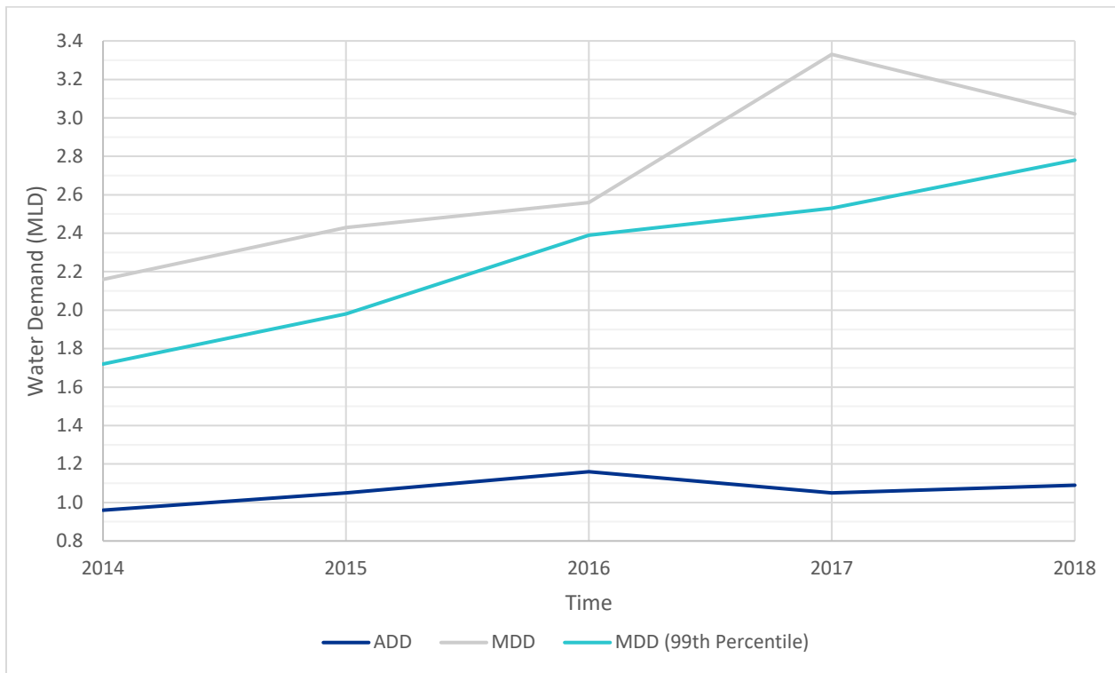
Figure 2-1 ADD and MDD from SCADA
