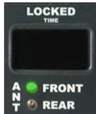
Figure 3.2.2.4b Antenna lights showing front antenna is active
