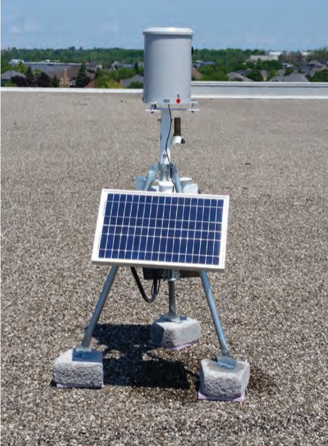
Figure 6 - Tipping Bucket Rain Gauge
