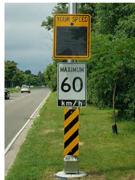
Modern radar speed board
