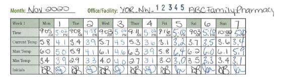
At least five (5) continuous business days of temperature recordings are required to demonstrate the vaccine refrigerator is working within the acceptable range of +2.0°C to +8.0°C prior to your inspection.
